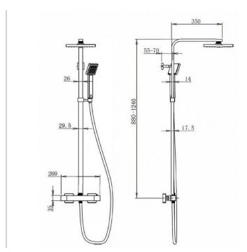
Dimensions are in millimetres except thread sizes which are BSP imperial.
