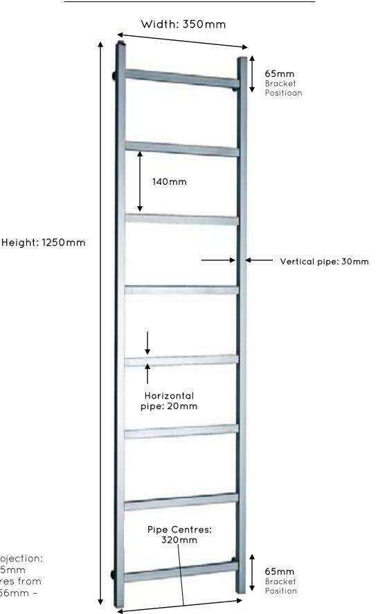
Overall Projection: 70mm - 95mm Pipe Centres from the Wall: 56mm -82mm
